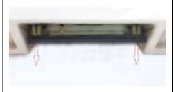
7. Push the switch back in with even pressure on both ends.
