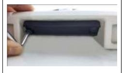
5. Be careful not to pull too much out to avoid damage the wire. The remove the cover and clean the surface.
